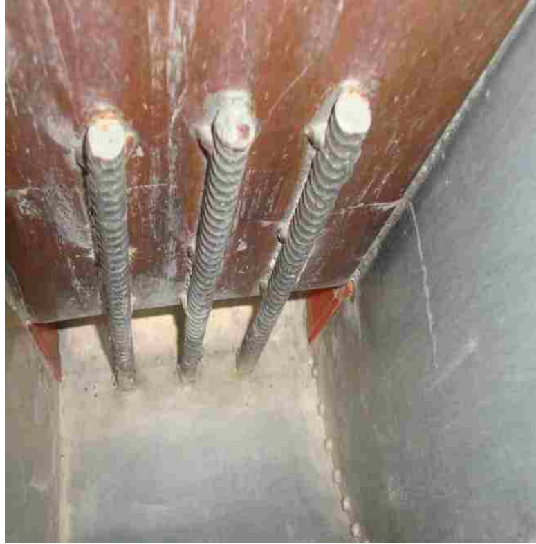
Figure 4.5: Rebar set-up in U-Box test apparatus
