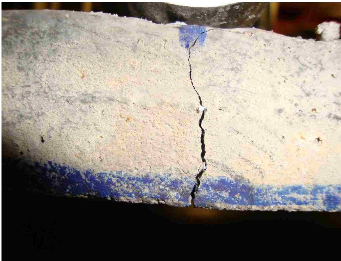
Figure 8.1.13: Failure patterns for long span 1% HSSFRC rectangular plates under transverse line load
