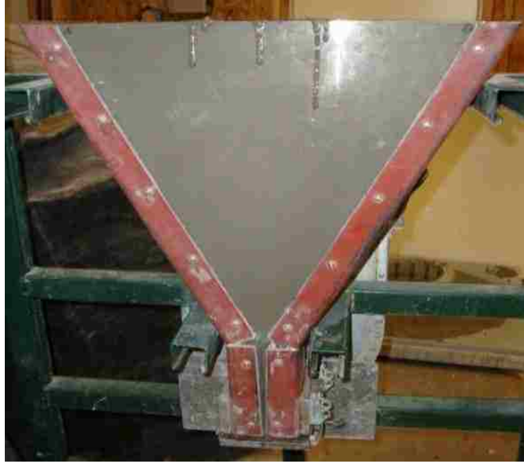
Figure 4.3: Typical V-Funnel test apparatus
