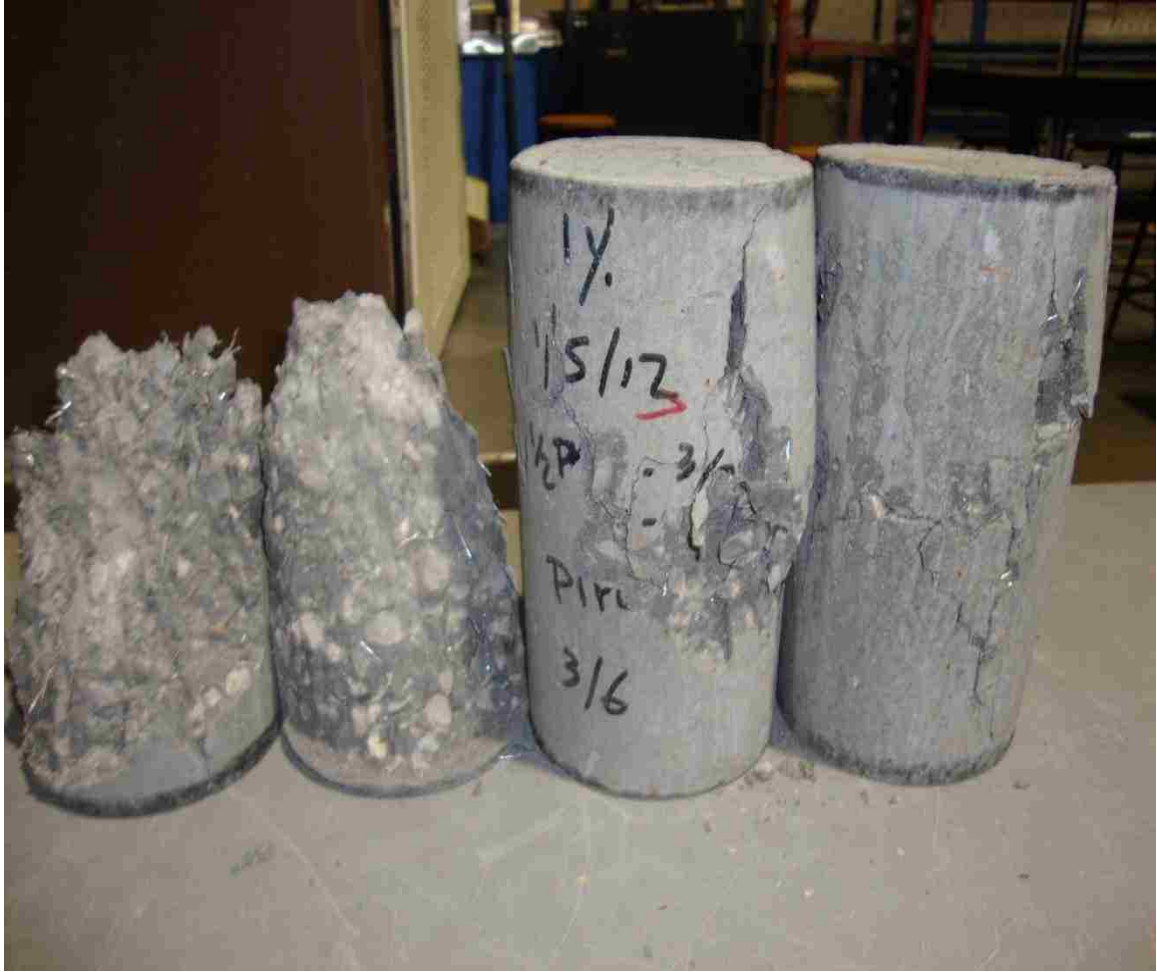
Figure 5.5: Failure mode for 1% HSSFRC cylinders under compression
