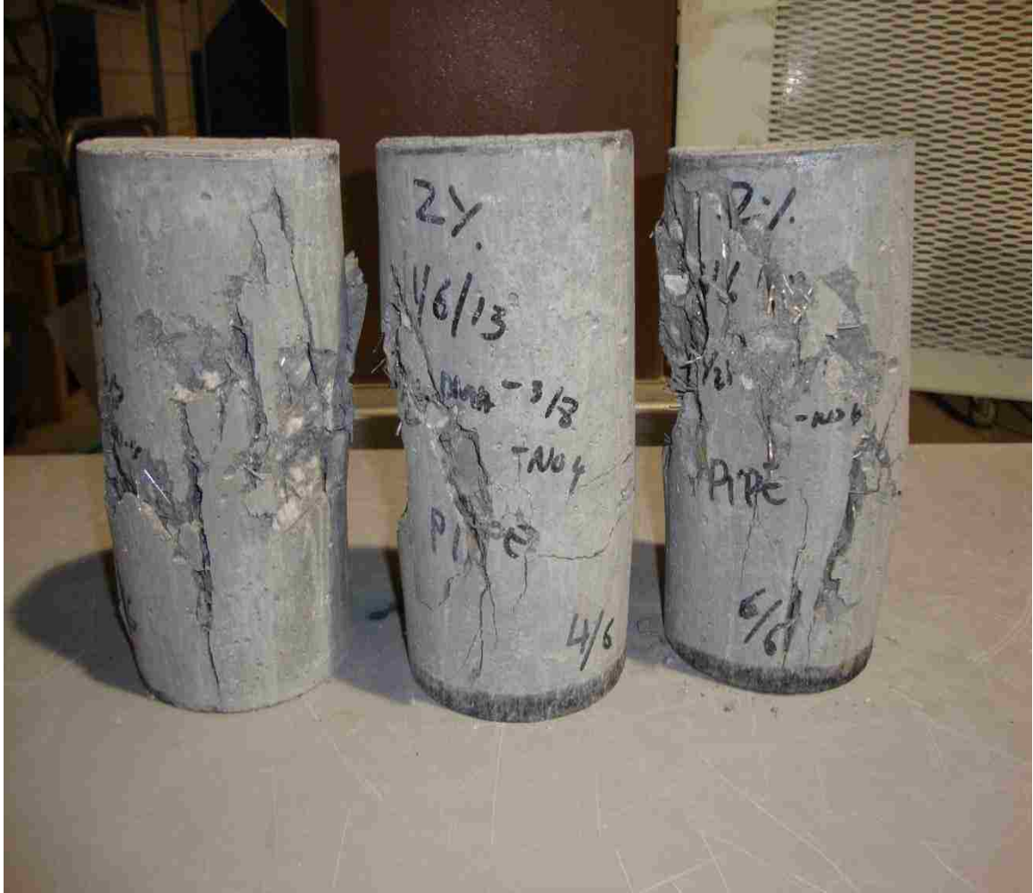
Figure 5.6: Failure mode for 2% HSSFRC cylinders under compression
