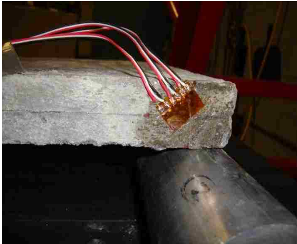
Figure 8.1.4: 45°- rectangular rosette at the support of HSSFRC rectangular plates (48 in. x 12 in.)
