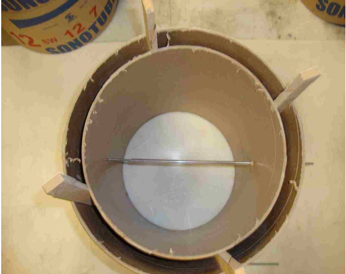
Figure 12.2: Formwork for circular cylindrical shells
