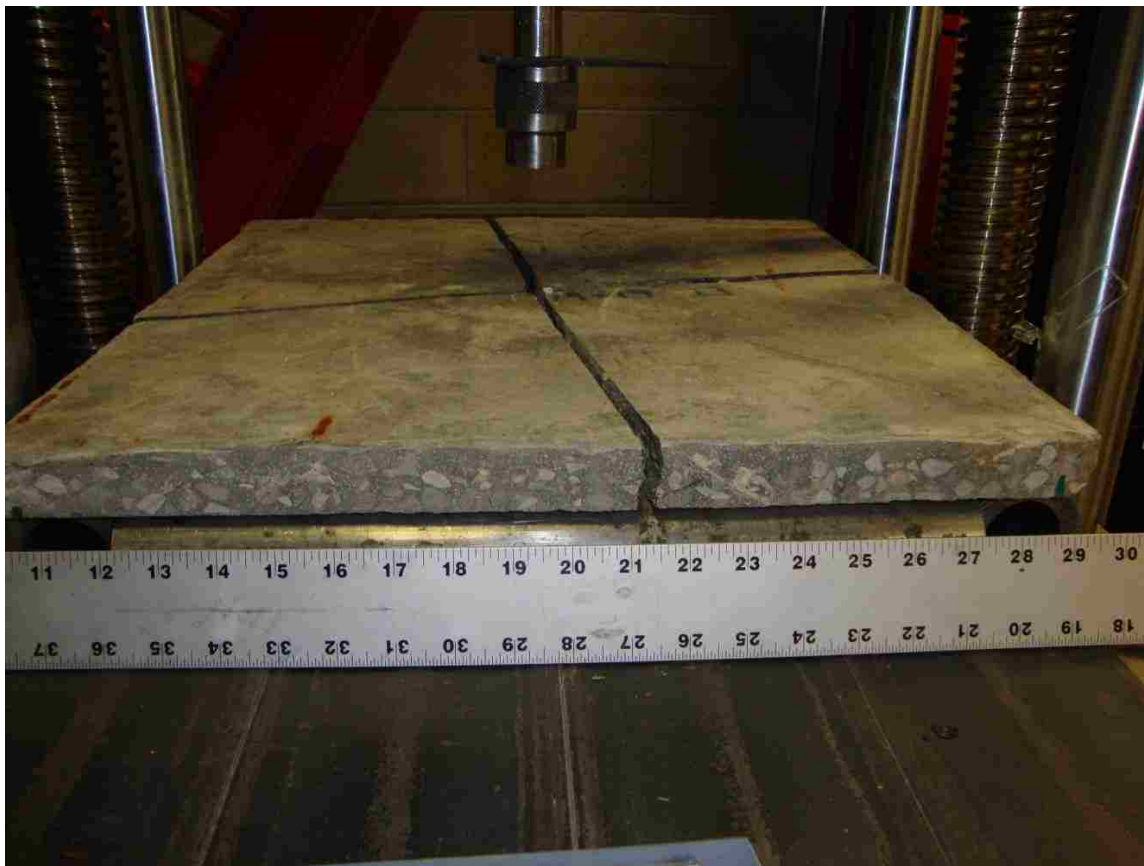
Figure 9.12: Failure patterns for 0% HSSFRC square plates under center point load
