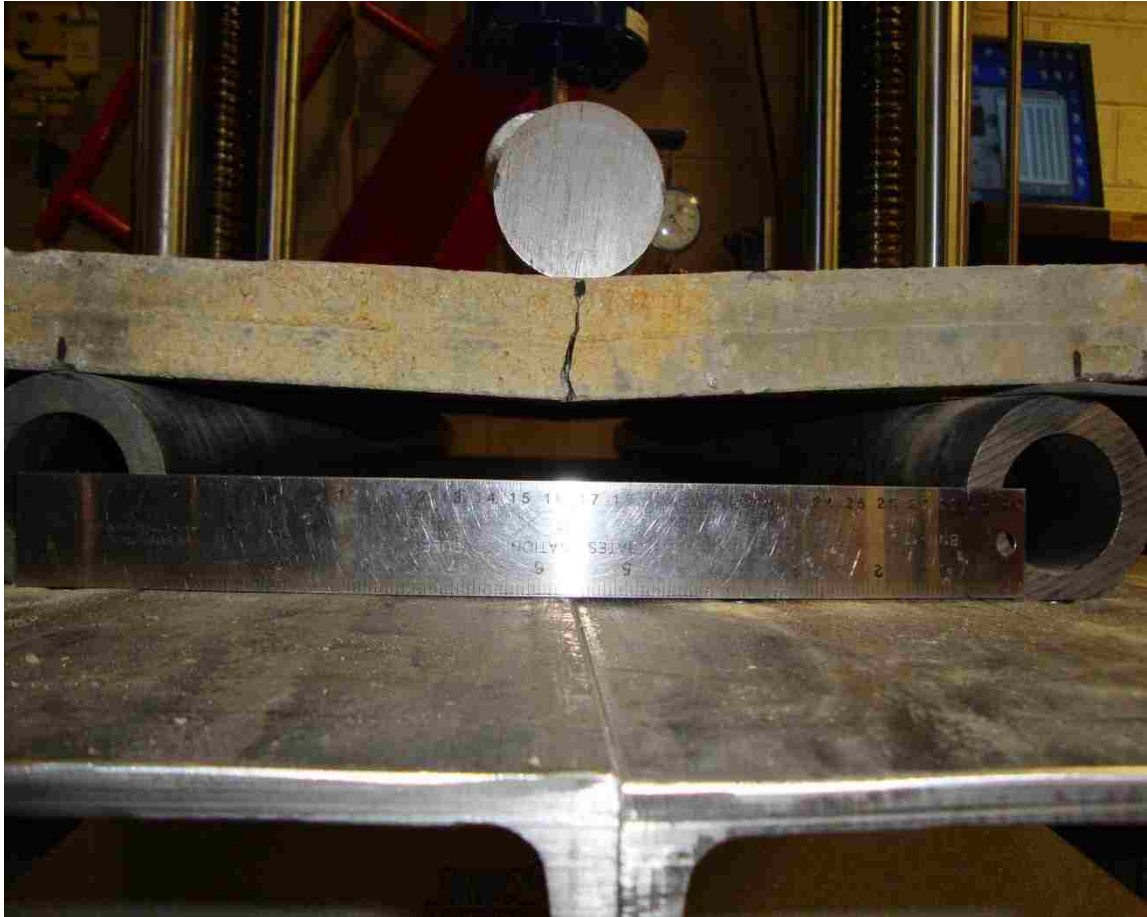
Figure 8.2.10: Failure patterns for short span 1% HSSFRC rectangular plates under longitudinal line load
