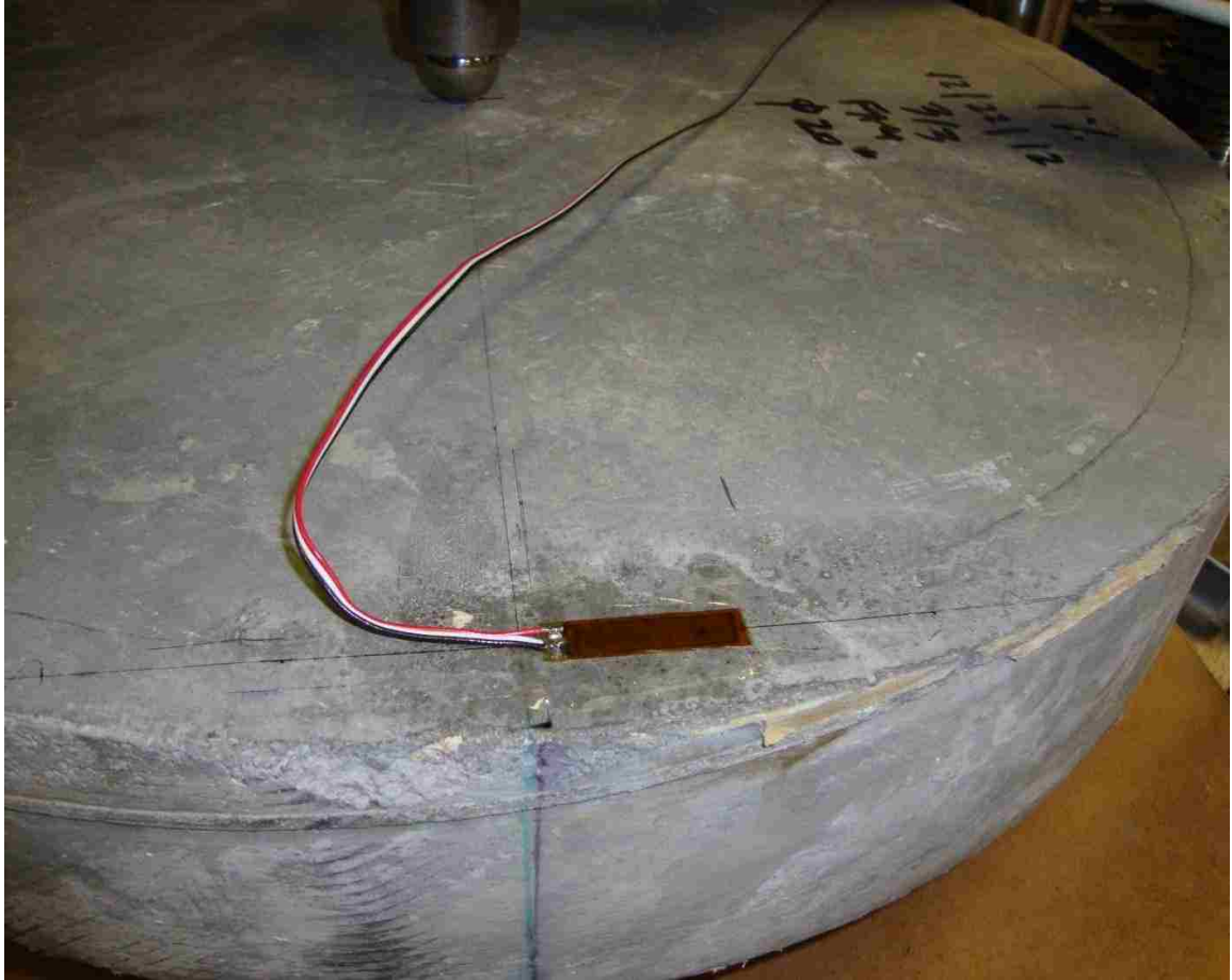
Figure 11.2: N2A-06-10CBE-350/E type strain gage located on the top surface of the circular plate and 3 mm (0.125 in.) away from the support point
