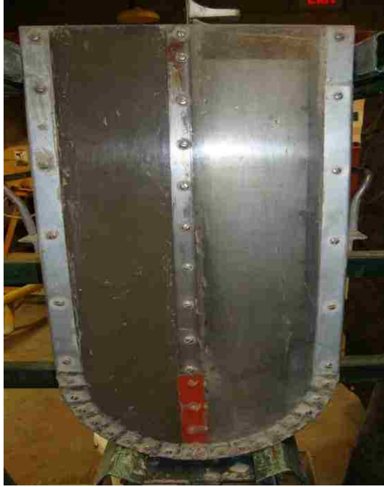
Figure 4.4: Typical U-Box test apparatus
