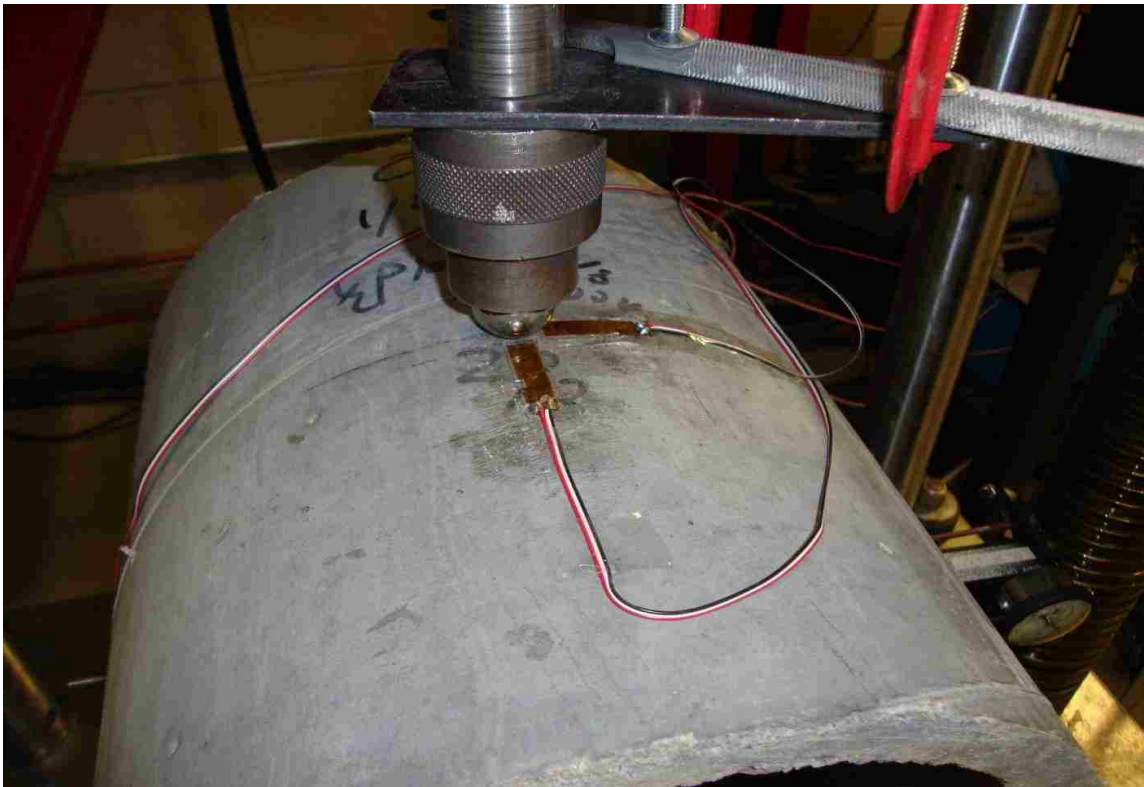
Figure 12.3: N2A-06-10CBE-350/E type strain gages located on the top surface of the circular cylindrical shell and 3 mm (0.125 in.) away from the center point load
