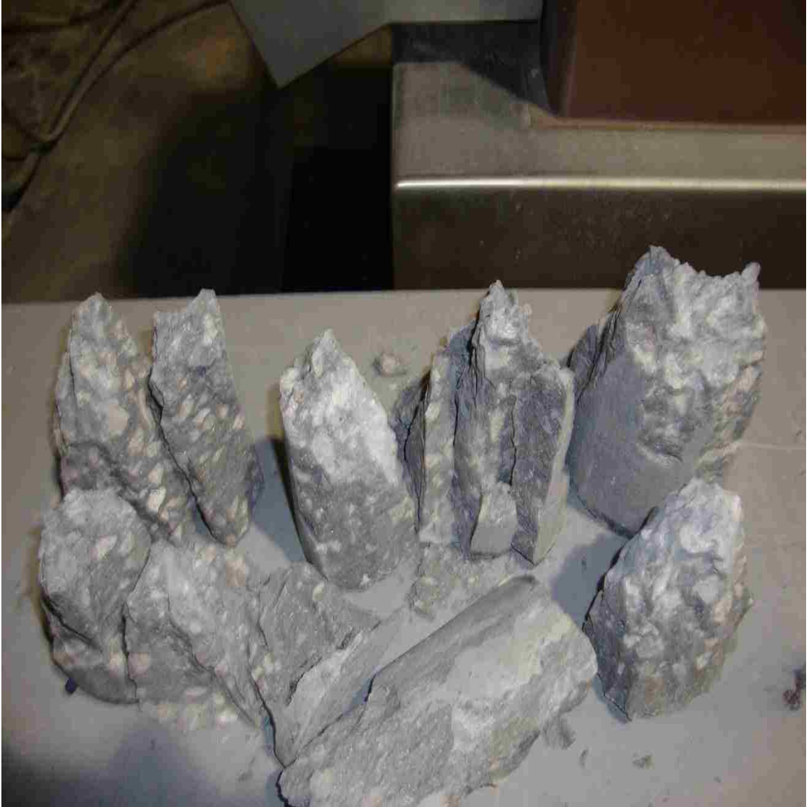
Figure 5.4: Failure mode for 0% HSSFRC cylinders under compression
