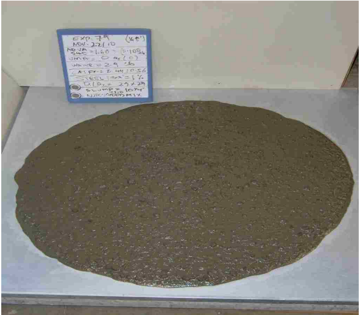
Figure 4.1: Typical SCC slump flow (spread diameter)
