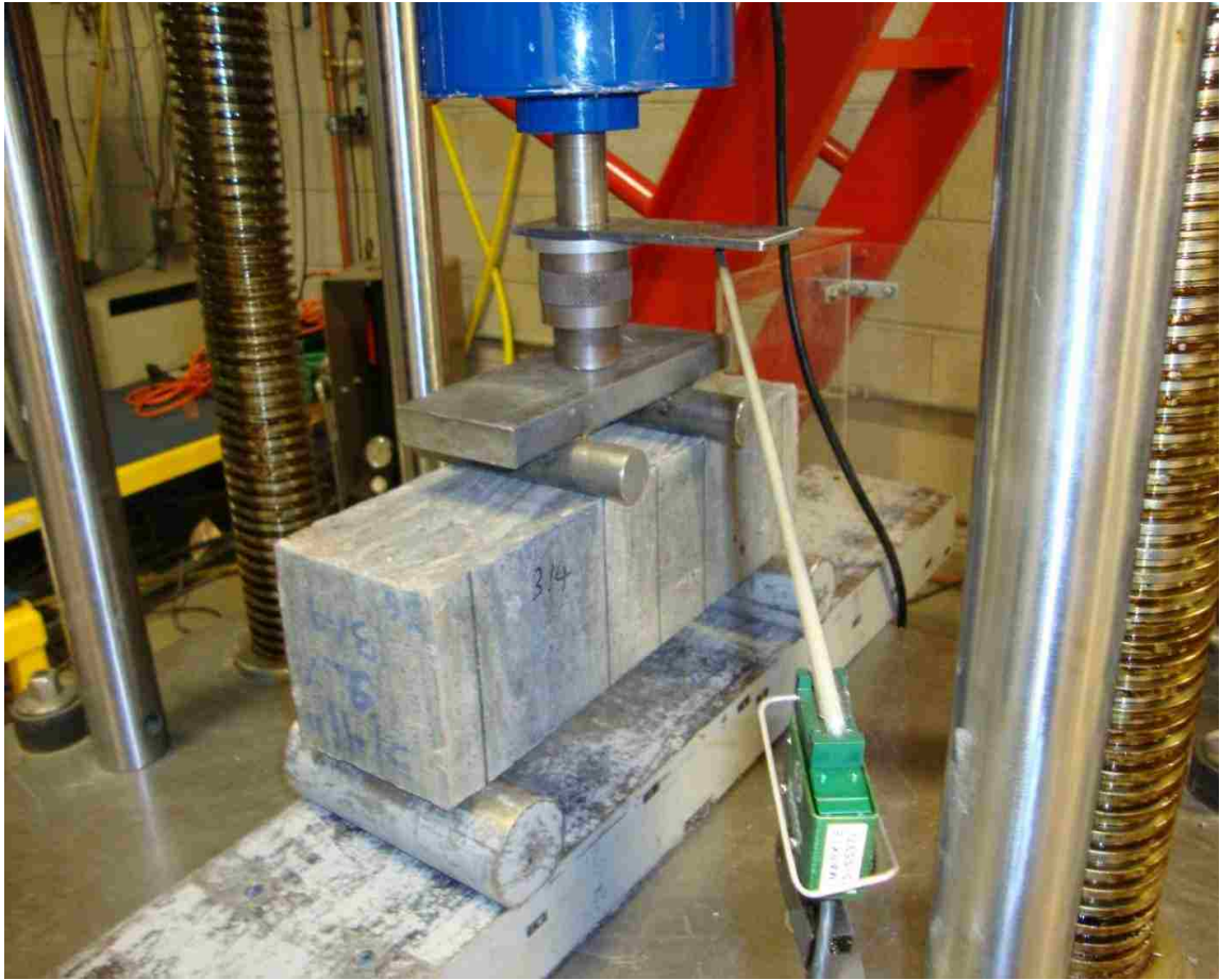
Figure 6.1: HSSFRC simple beam (4 in. x 4 in. x 12 in.) subjected to a third-point loading
