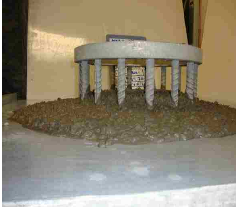
Figure 4.2: Typical J-Ring test apparatus
