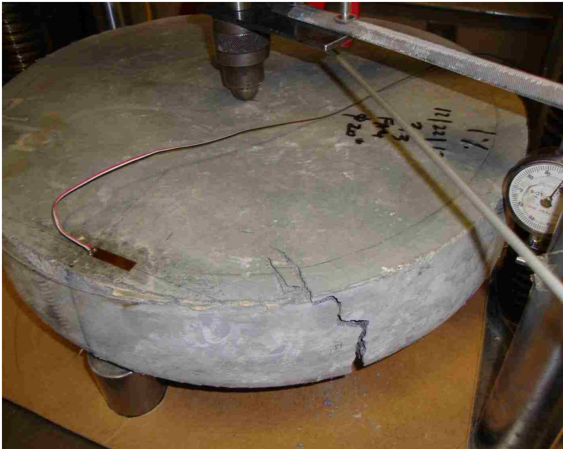
Figure 11.7: Test apparatus and specimen set up for circular plates under a concentrated center load
