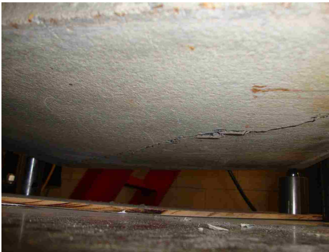
Figure 10.15: Crack pattern at the bottom surface for 1% HSSFRC square plates under concentrated opposite corner loads
